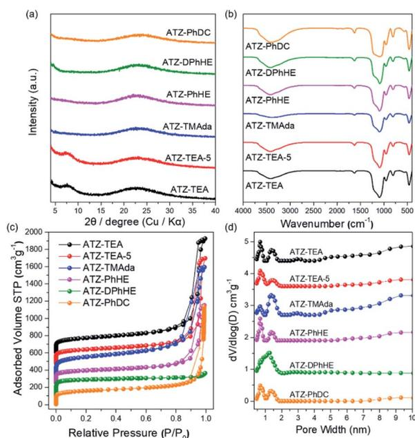
Fig. 1 (a) XRD patterns, (b) FT-IR spectra, (c) N<sub>2</sub> adsorption and desorption isotherms, and (d) pore size distributions of the ATZ samples.
