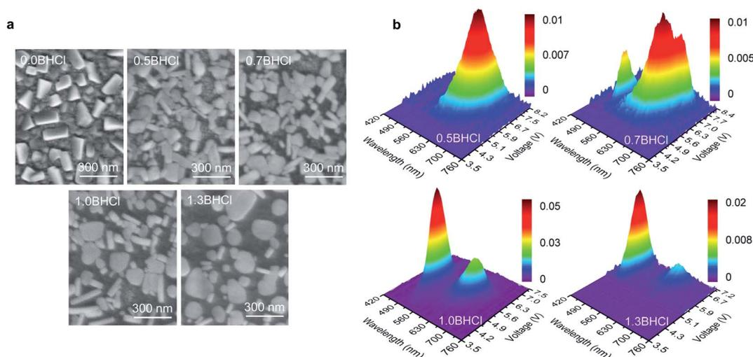
Fig. 3 (a) SEM images for  $m\text{BHCl}$  ( $m = 0.0, 0.5, 0.7, 1.0, \text{ and } 1.3$ ) films. (b) 3D surface images of EL spectra for devices based on  $m\text{BHCl}$  ( $m = 0.5, 0.7, 1.0, \text{ and } 1.3$ ) films.
