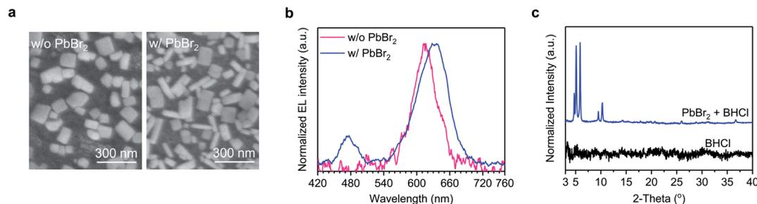
Fig. 4 (a) SEM images of perovskite films without and with PbBr<sub>2</sub>. (b) Normalized EL spectra of devices based on perovskite films without and with PbBr<sub>2</sub>. (c) XRD patterns of pure BHCl and PbBr<sub>2</sub> + BHCl mixed films.
