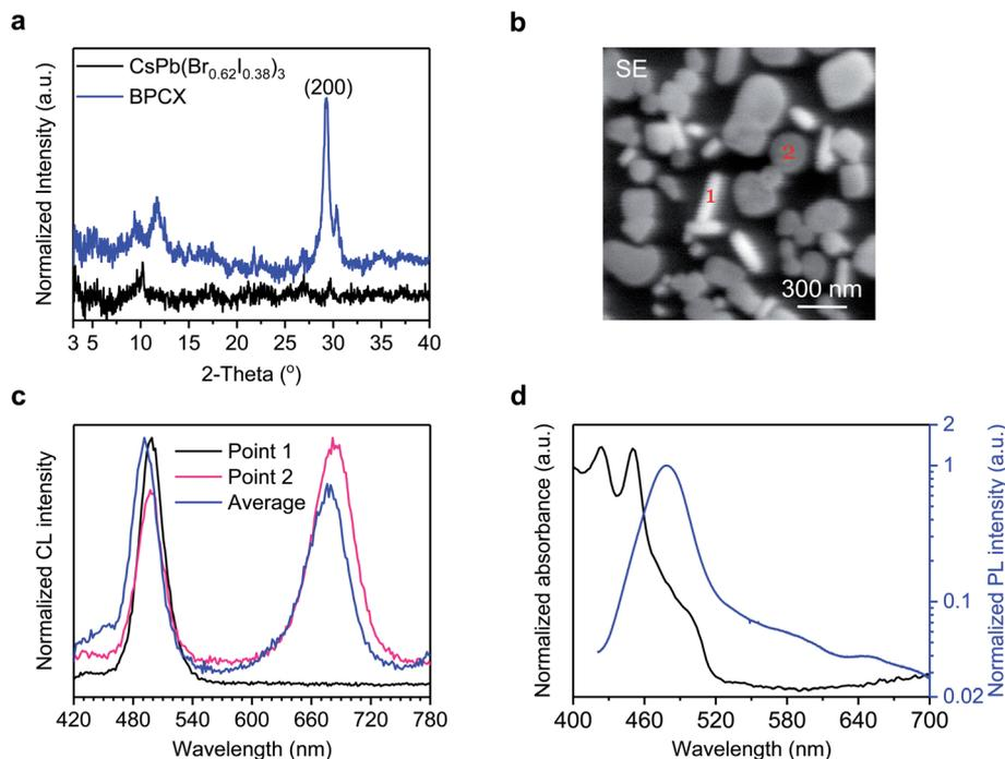
Fig. 2 (a) XRD patterns of  $\text{CsPb}(\text{Br}_{0.62}\text{I}_{0.38})_3$  and BCPX perovskite films. (b) Secondary electron (SE) image, and (c) cathodoluminescence (CL) spectra of the BCPX film acquired at 5.0 keV. (d) UV-vis absorption and PL spectra of the BCPX perovskite film.
