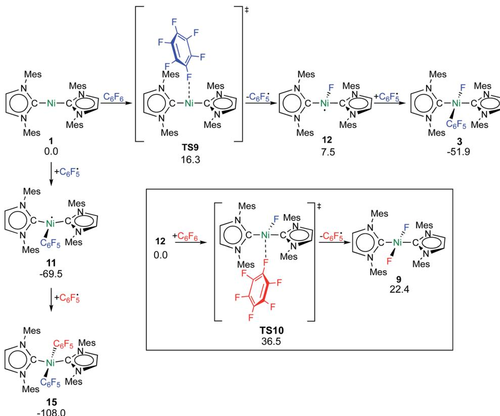
Scheme 10 Calculated pathways for the homolytic C–F bond cleavage of  $C_6F_6$  by **1** and further radical reaction steps ( $\Delta G^{298}$  in kcal mol $^{-1}$ ; energies of **TS10** and **9** are given relative to **12** +  $C_6F_6$ ).
