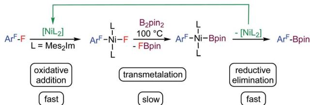
**Scheme 1** Thermal borylation of fluoroarenes with  $B_2pin_2$  mediated by  $[Ni(Mes_2Im)_2]$  via the oxidative addition product  $trans-[Ni(Mes_2Im)_2(F)(Ar^F)]$  as the resting state of the catalysis.
