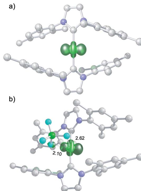
Fig. 5 (a) Spin density plot for  $[\text{Ni}(\text{Mes}_2\text{Im})_2]^+$ ; (b) molecular structure of  $\mathbf{8}_{\text{DFT1}}$  showing Ni– $\text{F}^{\text{BF}_4^-}$  contacts (isovalue  $\pm 0.0075\text{ a}_0^{-3}$ ; lengths of Ni–F contacts in  $\text{\AA}$ ; hydrogen atoms not shown).
