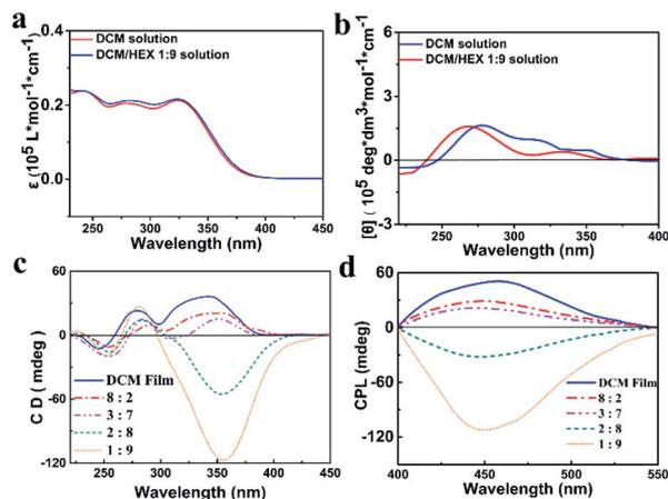
Fig. 2 Absorption spectra ( $5 \times 10^{-6}$  M) (a); CD spectra from solid films (c) and circularly polarized luminescence spectra (d) of *S*-TPE-Ph-PEA assemblies obtained from different solutions: DCM (blue); DCM/HEX 3 : 7 (cyan); DCM/HEX 2 : 8 (pink) and DCM/HEX 1 : 9 (red).
