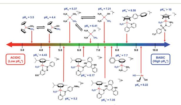
Fig. 3 Comparison of the  $pK_a$  values of aquated species of metal-based complexes.  $pK_a^*$  values refer to M-OD<sub>2</sub> complexes based on pH\* (pH meter reading not corrected for the effect of deuterium on the electrode).
