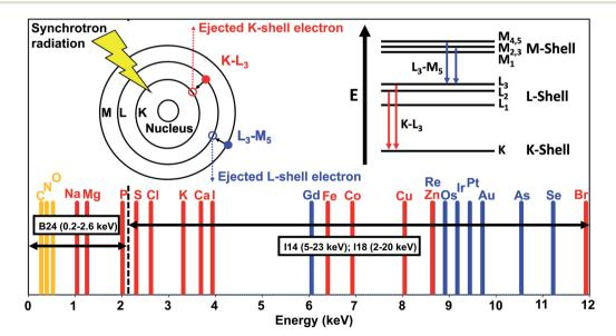
Fig. 11 Characteristic K-L $_3$  ( $2p_{3/2}^{-1} \rightarrow 1$  s $^{-1}$ ) and L $_3$ -M $_5$  ( $3d_{5/2}^{-1} \rightarrow 2p_{3/2}^{-1}$ ) X-ray fluorescence emissions. K-L $_3$  for elements exploited in cryosoft-X-ray tomography are in yellow, abundant endogenous elements in red; L $_3$ -M $_5$  of exogenous elements are blue. Additional elements are reported in Table S11† B24 and I14 refer to beamlines at the Diamond synchrotron (www.diamond.ac.uk).
