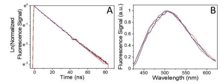
Fig. 1 (A) normalized fluorescence decay of 4F-9AC crystals before (black) and after (red) exposure to 405 nm light that reacts  $\sim 50\%$  of the sample. The solid blue line is a single exponential fit with a lifetime of 27 ns. (B) The normalized fluorescence spectrum at 10 ns, 20 ns, and 40 ns delays. The single exponential decay and lack of spectral evolution are consistent with a single emitting species. There is no sign of chemical damage after 50% photodimerization.
