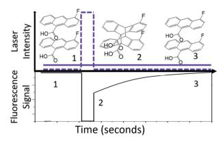
Fig. 2 Fluorescence-recovery-after-photobleaching (FRAP) experimental design. The top figure shows how the "bleach" (dashed) and "probe" (solid) beam intensities change with time as well as the corresponding dimerization and relaxation of 4F9AC. The bottom figure shows the dominant species in each time regime and the expected fluorescence signal recovery after the bleach pulse.
