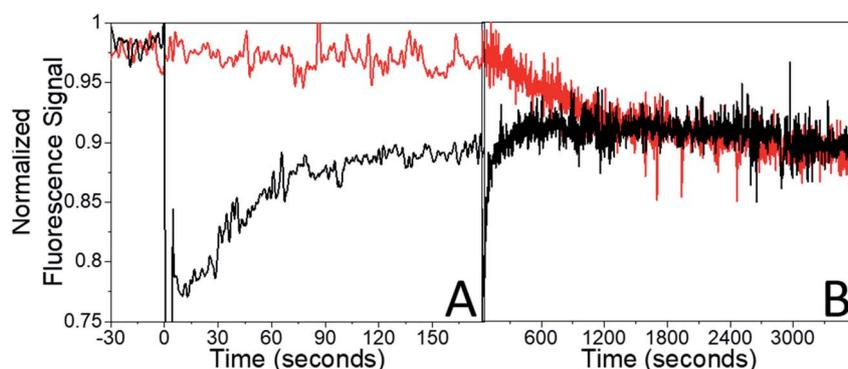
Fig. 7 (A) Early time fluorescence recovery curves for a 30% bleach (black) compared to a control signal with no pump pulse. Over the timescale of 180 seconds, there appears to be no change in the control signal. (B) Long time fluorescence signals for the 30% bleach and control signals, where they converge after  $\sim 1$  h.
