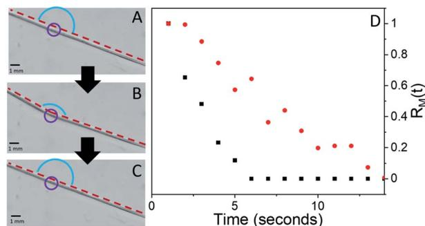
Fig. 5 Microscope images of single **4F-9AC** microneedle (A) before UV pulse, (B) 2 s after UV pulse, (C) 30 s after UV pulse. The photo-mechanical motion can be seen in (A–C) showing bending and unbending of the crystal. (D) Bend recovery function  $R_M(t)$  for two different UV pulse durations (1 second (black) and 5 seconds (red)).
