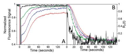
Fig. 3 (A) Fluorescence recovery signal as a function of bleach depth, which is controlled through pump pulse durations of 0.5 s (black), 2 s (green), 3 s (pink), 4 s (blue), and 5 s (red). B)  $R_F(t)$  initial bleach decays for the different change in the intrinsic recovery with respect to the different pump pulse durations, taking into account the lack of full recovery.
