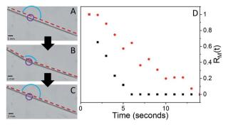
Fig. 5 Microscope images of single 4F-9AC microneedle (A) before UV pulse, (B) 2 s after UV pulse, (C) 30 s after UV pulse. The photomechanical motion can be seen in (A–C) showing bending and unbending of the crystal. (D) Bend recovery function  $R_{\rm M}(t)$  for two different UV pulse durations (1 second (black) and 5 seconds (red)).
