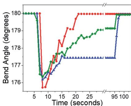
Fig. 6 Different photomechanical recoveries from the same UV bending pulse and different hold beam strengths: no hold beam (red), 1.25  $\mu\text{W}$  (green), 2.5  $\mu\text{W}$  (blue). At 100 seconds, the hold beams are blocked, and the bend quickly recovers.
