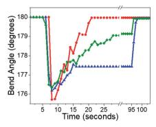
Fig. 6 Different photomechanical recoveries from the same UV bending pulse and different hold beam strengths: no hold beam (red), 1.25  $\mu$ W (green), 2.5  $\mu$ W (blue). At 100 seconds, the hold beams are blocked, and the bend quickly recovers.
