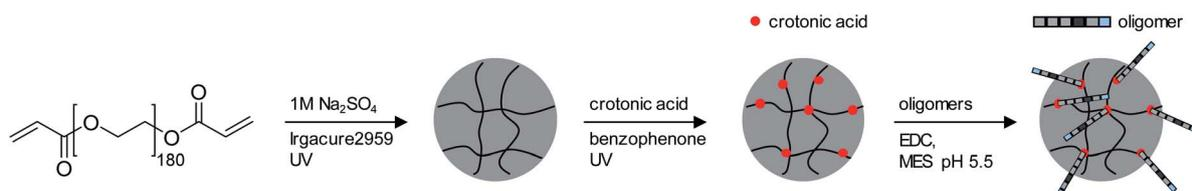
Fig. 4 Synthesis of PEG based SCPs. (1) liquid–liquid phase separation of PEG macromonomers in 1 M NaSO $_4$  followed by UV crosslinking; (2) photochemical grafting of crotonic acid using benzophenone; (3) coupling of oligomers by carbodiimide chemistry.
