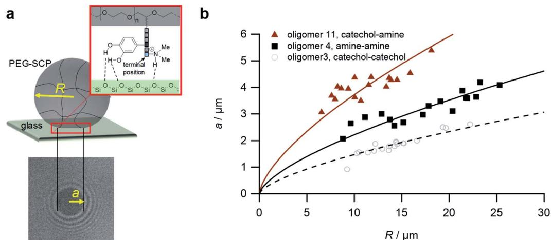
Fig. 5 The SCP adhesion assay. (a) Schematic representation of an oligomer-functionalized SCP adhering to a glass slide. The reflection interference contrast microscopy image (bottom) shows a typical contact area (dark area in the center) and newton rings providing the geometry of the SCP, *i.e.* the parameters  $a$  and  $R$ . (b) Typical JKR plots and fits (lines) according to eqn (1) depicting the oligomers **3** (empty circles), **4** (squares) and **11** (triangles).
