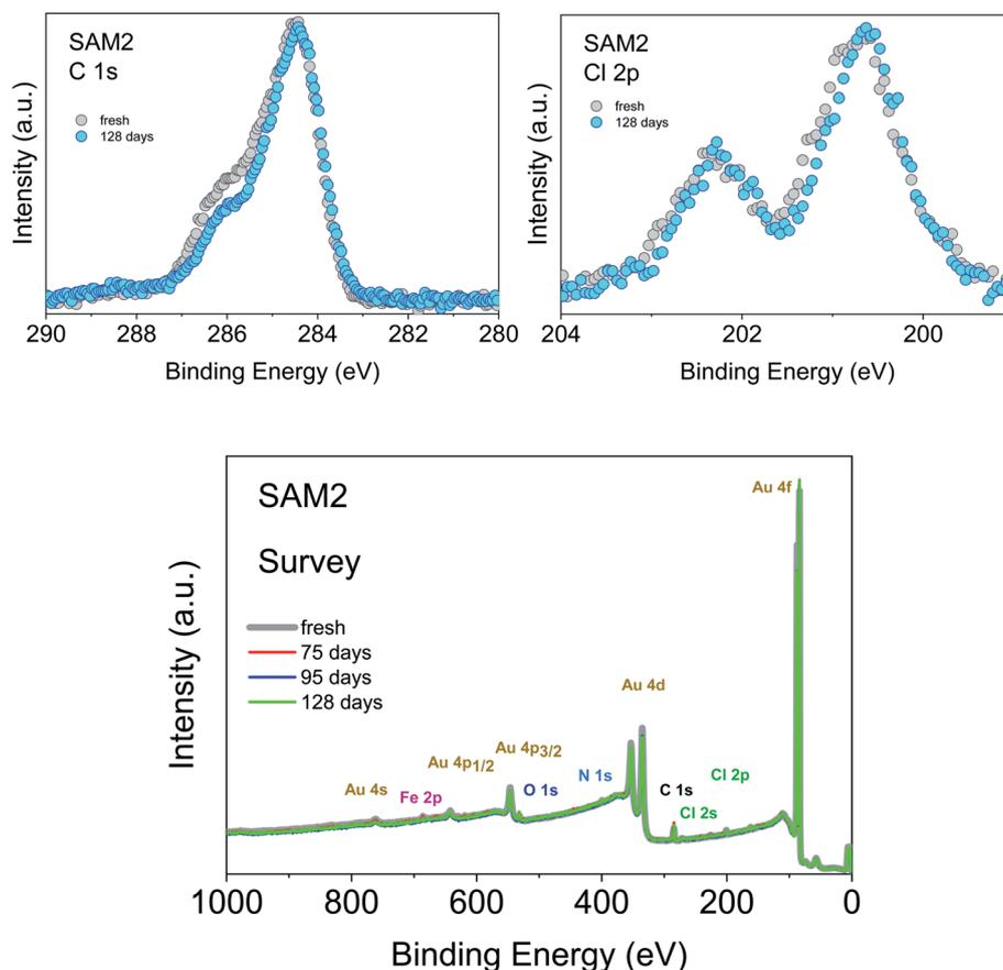
Fig. 5 Upper panel: (left) C 1s and (right) Cl 2p core level spectra of a freshly prepared monolayer and after 128 days of exposure to air and kept in darkness, as indicated (photon energy: 1486.6 eV). Intensities are normalized to the peak maximum to allow comparison. Lower panel: SAM2 survey XPS spectra under air exposure, as indicated (photon energy: 1486.6 eV).
