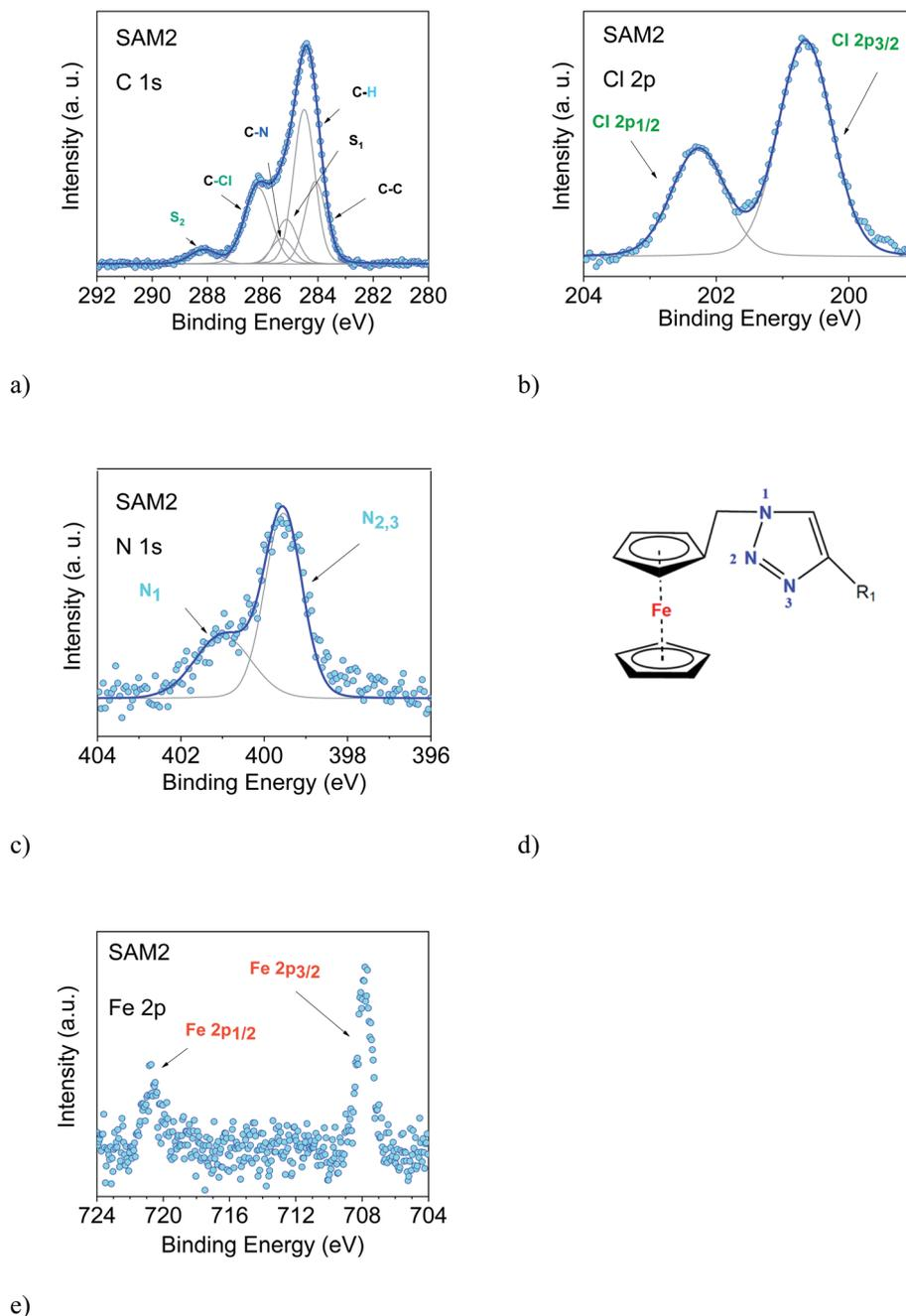
Fig. 2 SAM2. (a) C 1s, (b) Cl 2p, (c) N 1s (together with their best fit) and (e) Fe 2p XPS spectra (photon energy: 1486.6 eV). In (d) the chemical environment of the triazole derivative is shown in detail.
