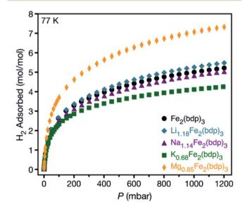
Fig. 4 Hydrogen adsorption isotherms for microcrystalline powder samples of neutral and reduced variants of  $Fe_2(bdp)_3$  collected at 77 K.
