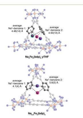
Fig. 2 Single-crystal X-ray structures of  $Na_2Fe_2(bdp)_3 \cdot yTHF$  (top) and activated  $Na_{0.5}Fe_2(bdp)_3$  (bottom), highlighting the interactions between the inserted cations and the benzene rings of the ligands. The disordered sites of  $Na^+$  are highlighted in red, blue, and green. Orange, purple, blue, and gray spheres represent Fe, Na, N, and C atoms, respectively; H atoms and symmetry-generated  $Na^+$  are omitted for clarity.
