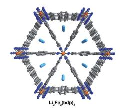
Fig. 3 Single-crystal X-ray structures of activated  $\text{Li}_2\text{Fe}_2(\text{bdp})_3$ . Orange, light blue, blue, and gray spheres represent Fe, Li, N, and C atoms, respectively; H atoms are omitted for clarity.
