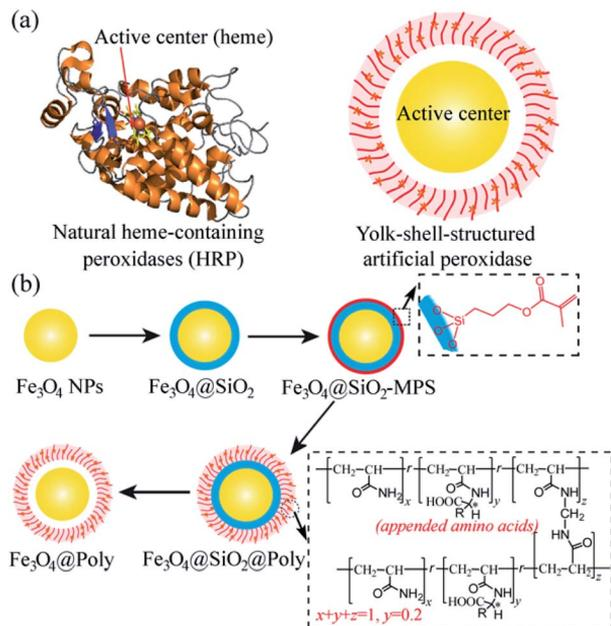
**Scheme 1** (a) Representative structures of natural heme-containing peroxidase (left) and yolk-shell-structured artificial peroxidase (right). (b) Preparation procedures of the yolk-shell-structured artificial peroxidase.
