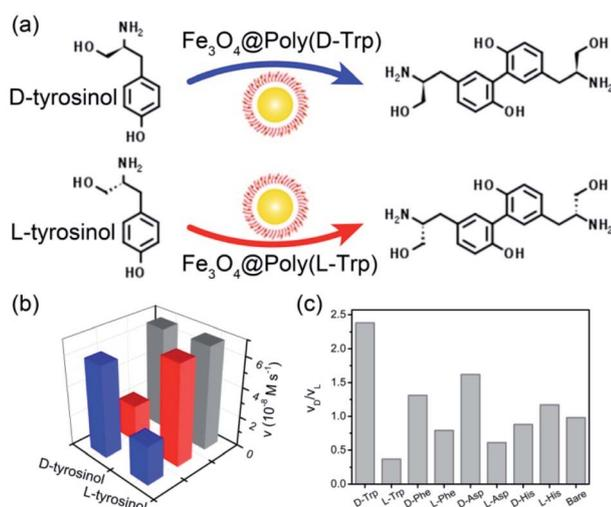
Fig. 2 (a) The enantioselective oxidation of chiral tyrosinol catalyzed by  $\text{Fe}_3\text{O}_4@\text{Poly(L-/D-Trp)}$ . (b) The initial velocity for the oxidation of tyrosinol enantiomers with  $\text{Fe}_3\text{O}_4@\text{Poly(D-Trp)}$  (blue),  $\text{Fe}_3\text{O}_4@\text{Poly(L-Trp)}$  (red) and bare  $\text{Fe}_3\text{O}_4$  (gray). (c) The ratio of initial rates for the oxidation of the *D* enantiomer to *L* enantiomer.
