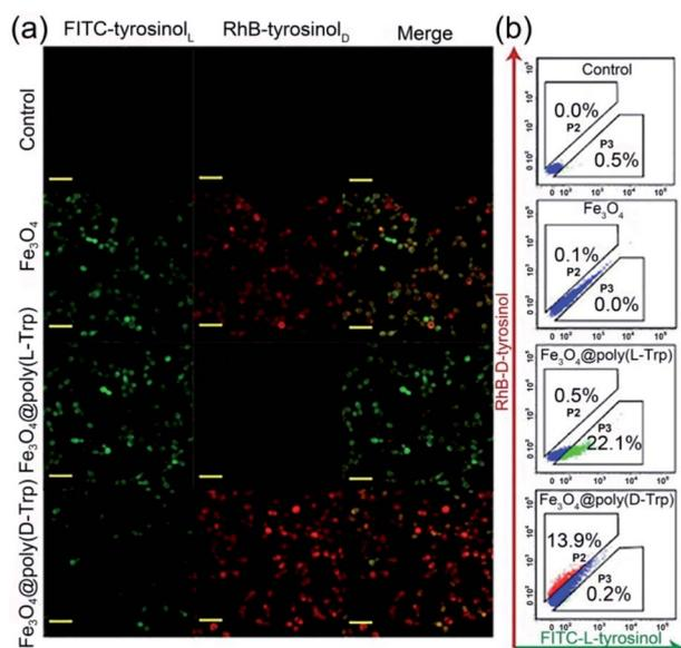
Fig. 4 (a) Confocal fluorescence microscopy and (b) flow cytometry analysis results of yeast cells treated with H<sub>2</sub>O<sub>2</sub> (100 μM), FITC-tyrosinol<sub>L</sub> and RhB-tyrosinol<sub>D</sub> with no nanozyme (control), bare Fe<sub>3</sub>O<sub>4</sub>, Fe<sub>3</sub>O<sub>4</sub>@Poly(*L*-Trp) or Fe<sub>3</sub>O<sub>4</sub>@Poly(*D*-Trp), respectively. (Scale bars: 20 μm.)
