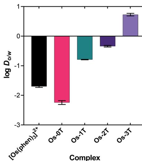
Fig. 2 Octanol-water distribution coefficients ( $\log D_{o/w} \pm \text{SD}$ ) for reference compound  $[\text{Os}(\text{phen})_3]^{2+}$  and **Os-0T-Os-3T** ( $\text{Cl}^-$  salts); SD = standard deviation. The value of  $\log D_{o/w}$  for **Os-4T** could not be determined due to its precipitation from the solvent mixture.
