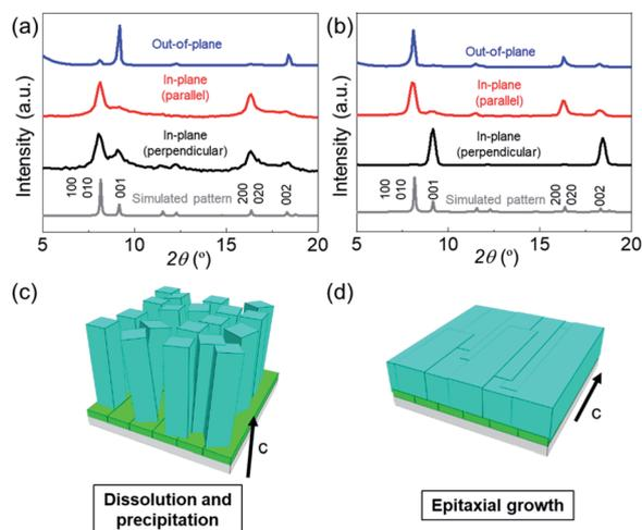
Fig. 3 XRD patterns and the corresponding schematics of the  $\text{Cu}_2(1,4\text{-NDC})_2\text{DABCO}$  film synthesized at 16 mM 1,4- $\text{H}_2\text{NDC}$  and 4 mM DABCO (a and c), and 16 mM 1,4- $\text{H}_2\text{NDC}$  and 1024 mM DABCO (b and d). Three setups for the XRD investigations were used: out-of-plane (blue line) and in-plane (red and black lines, where the X-ray incident angle is parallel and perpendicular to the longitudinal direction of the nanobelts at  $2\theta = 0^\circ$ ).
