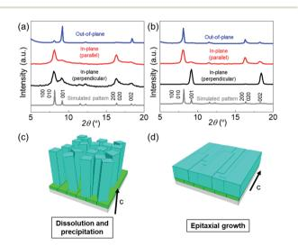
Fig. 3 XRD patterns and the corresponding schematics of the Cu<sub>2</sub>(1,4-NDC)<sub>2</sub>DABCO film synthesized at 16 mM 1,4-H<sub>2</sub>NDC and 4 mM DABCO (a and c), and 16 mM 1,4-H2NDC and 1024 mM DABCO (b and d). Three setups for the XRD investigations were used: out-ofplane (blue line) and in-plane (red and black lines, where the X-ray incident angle is parallel and perpendicular to the longitudinal direction of the nanobelts at  $2\theta = 0^{\circ}$ ).
