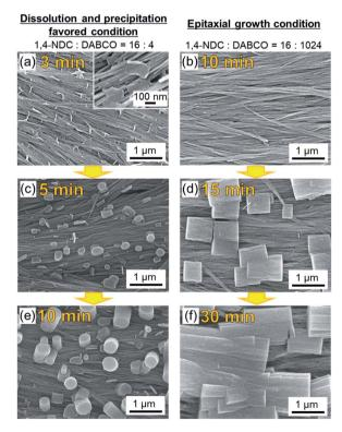
Fig. 4 Evolution of the MOF growth under each set of conditions. SEM images of Cu<sub>2</sub>(1,4-NDC)<sub>2</sub>DABCO films synthesized under the conditions favouring dissolution and precipitation with varied reaction time (left): 3 (a), 5 (c), and 10 min (e). SEM images of  $Cu_2(1,4-NDC)_2DABCO$ films synthesized under the epitaxial growth conditions with varied reaction time (right): 10 (b), 15 (d), and 30 min (f).
