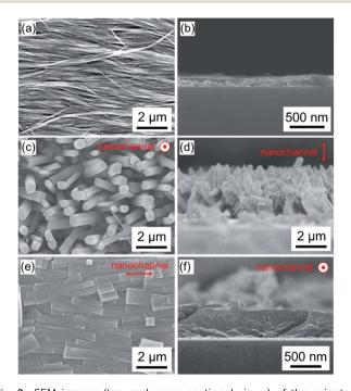
Fig. 2 SEM images (top and cross-sectional views) of the oriented Cu(OH)2 nanobelt film (a and b) and Cu2(1,4-NDC)2DABCO films synthesized under different conditions: 16 mM 1,4-H2NDC and 4 mM DABCO (c and d), and 16 mM 1,4-H<sub>2</sub>NDC and 1024 mM DABCO (e and f). The out-of-focus object observed on the back of the Cu<sub>2</sub>(1,4-NDC)<sub>2</sub>DABCO film in part (f) is carbon tape which was used to prepare the samples for cross-sectional SEM.
