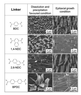
Fig. 6 SEM images of  $Cu_2(linker)_2DABCO$  (linker = BDC, 1,4-NDC, 2,6-NDC, and BPDC) oriented films under the conditions favouring dissolution and precipitation, and epitaxial growth.
