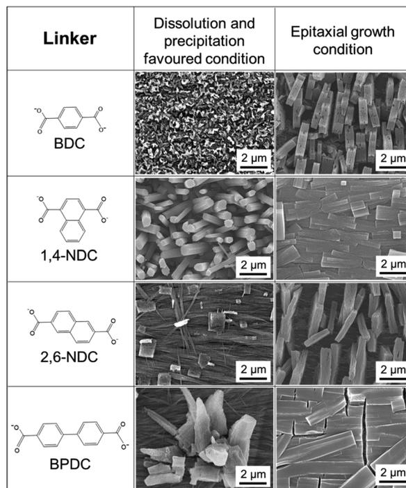
Fig. 6 SEM images of  $\text{Cu}_2(\text{linker})_2\text{DABCO}$  (linker = BDC, 1,4-NDC, 2,6-NDC, and BPDC) oriented films under the conditions favouring dissolution and precipitation, and epitaxial growth.
