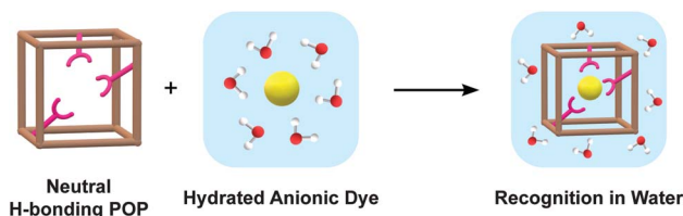
Fig. 1 Cartoon schematic illustrating the approach used in this study to bind anionic dyes (yellow sphere) in water with a porous organic polymer host (brown cube) with neutral hydrogen (H) bonding functional groups (pink receptor). Water molecules are shown as red (oxygen atom) and white (hydrogen atom) spheres in the blue background to represent the aqueous environment.
