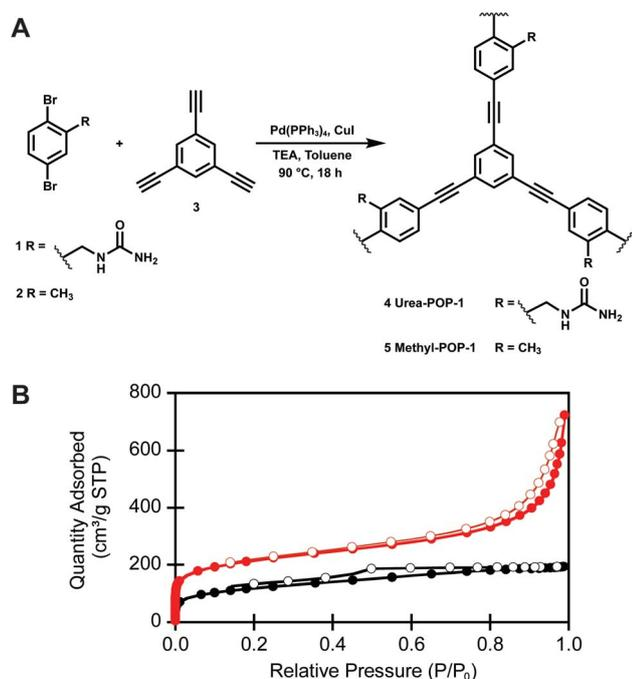
Fig. 2 (A) Synthesis of Urea-POP-1 and Methyl-POP-1 through a Sonogashira polymerization. (B) Representative nitrogen adsorption (closed circles) and desorption (open circles) isotherms Urea-POP-1 (red) and Methyl-POP-1 (black).
