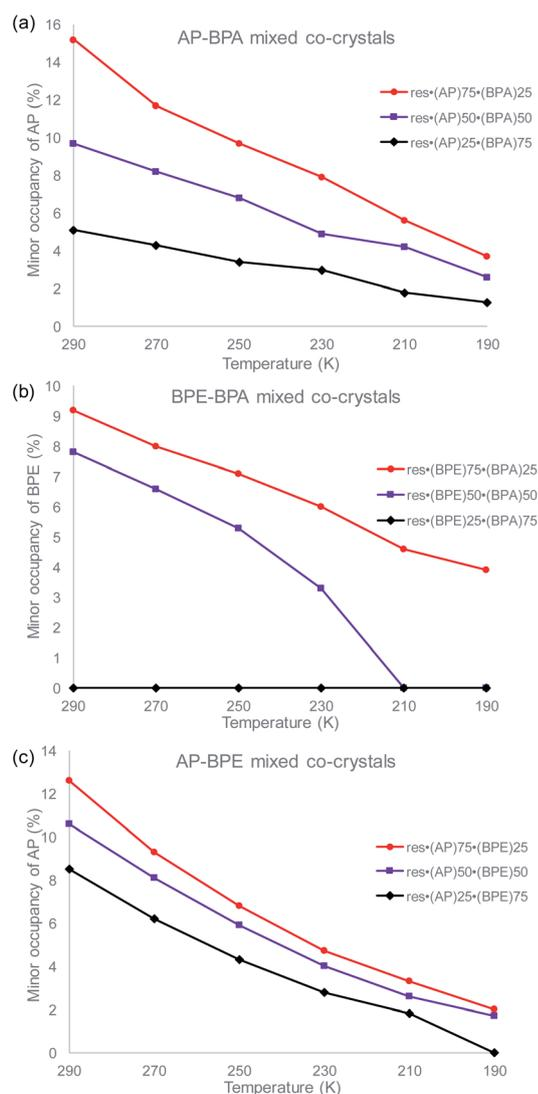
Fig. 2 Change in the minor site occupancies of the motion-capable group as a function of temperature for: (a)  $\text{res}\cdot(\text{AP})_x\cdot(\text{BPA})_y$ , (b)  $\text{res}\cdot(\text{BPE})_x\cdot(\text{BPA})_y$ , and (c)  $\text{res}\cdot(\text{AP})_x\cdot(\text{BPE})_y$ .
