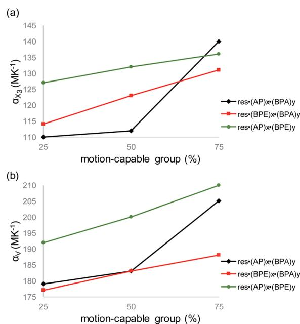
Fig. 4 Variation in (a) TE coefficient along  $X_3$  and (b) volumetric TE coefficient as a function of the amount of motion-capable molecule within the mixed cocrystals. For res·(AP)<sub>x</sub>·(BPE)<sub>y</sub>, the motion-capable group (plotted along the x-axis) refers to AP.
