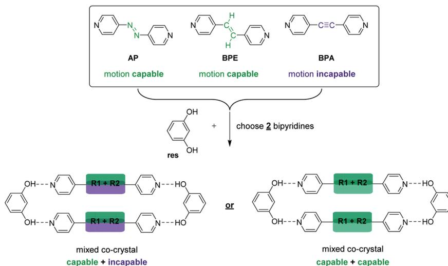
Scheme 3 Components and synthesis of mixed cocrystals.
