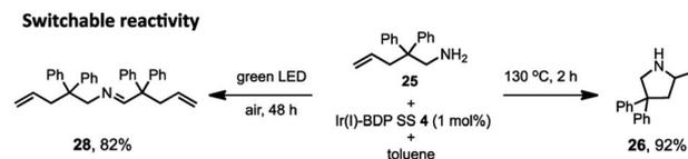
Scheme 5 The switchable reactivity of compound **25**, where heat leads to generation of compound **26** (right) and light irradiation produces compound **28** (left). Conditions: aminoalkene **25** (0.4 mmol), catalyst **4** (0.004 mmol), toluene (2 mL). Either heated under argon to give product **26**, or irradiated under air to give product **28**. Conversion determined using  $^1\text{H}$  NMR spectroscopy, relative to the internal standard 2,4,6-trimethoxybenzene (0.4 mmol).
