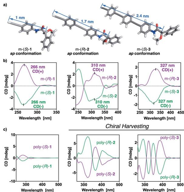
Fig. 4 (a) X-ray structures of *m*-(*S*)-1, *m*-(*R*)-2 and *m*-(*S*)-3. (b) CD traces of *m*-(*S*)- and *m*-(*R*)-1; *m*-(*S*)- and *m*-(*R*)-2; *m*-(*S*)- and *m*-(*R*)-3 in  $\text{CHCl}_3$  ( $0.1 \text{ mg mL}^{-1}$ ). (c) CD spectra for poly-(*S*)- and poly-(*R*)-1 in  $\text{CHCl}_3$  ( $0.1 \text{ mg mL}^{-1}$ ); poly-(*S*)- and poly-(*R*)-2 in DMSO ( $0.1 \text{ mg mL}^{-1}$ ); poly-(*S*)- and poly-(*R*)-3 in DMSO ( $0.1 \text{ mg mL}^{-1}$ ).
