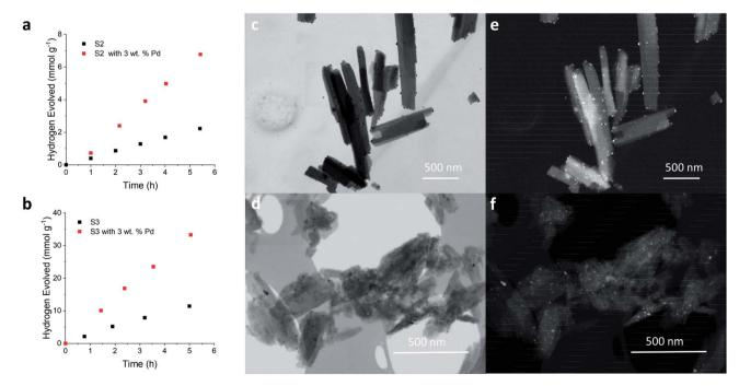
Fig. 4 Hydrogen evolution of (a) S2 (5 mg) and (b) S3 (5 mg) in TEA/MeOH/water (1 : 1 : 1, 5 mL) with and without the addition of 3 wt% Pd by photodeposition of [Pd(NH<sub>4</sub>)<sub>2</sub>Cl<sub>4</sub>], irradiated with a 300 W Xe light source fitted with a  $\lambda > 295$  nm filter. STEM images of S2 with 3 wt% Pd in (c) bright field mode and (e) high angle dark field mode and S3 with 3 wt% Pd in (d) bright field mode and (f) high angle dark field mode.
