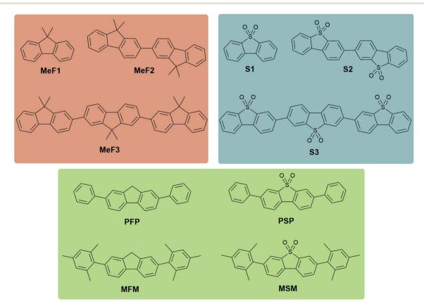
Fig. 1 Structures of the oligomer photocatalysts in this study.
