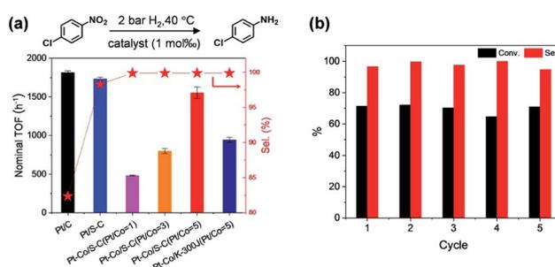
Fig. 6 Catalytic performance of Pt-Co bimetallic NPs for nitroarene hydrogenation. (a) TOF and selectivity for *p*-chloroaniline of Pt-Co/S-C and reference catalysts. (b) Recycling experiments over five runs for Pt-Co/S-C (Pt/Co = 5). Note that the selectivity (a) and recycling experiments (b) were chosen at 2.0 h and 30 min, respectively. Reaction conditions: 3 mmol substrate, 1 mol% Pt catalyst, methyl alcohol, 2 bar H<sub>2</sub>, 40 °C.
