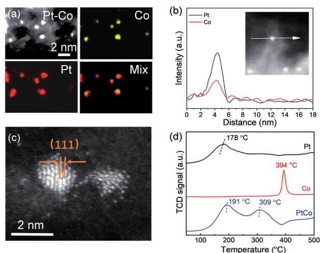
Fig. 3 Characterization of Pt–Co bimetallic NPs on S–C. (a) EDS elemental mapping. (b) EDS line scan. (c) Atomic resolution HAADF-STEM image. (d) TPR of monometallic Pt and Co and bimetallic Pt–Co on the S–C supports.
