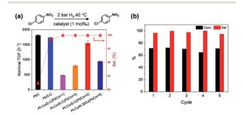
Fig. 6 Catalytic performance of Pt-Co bimetallic NPs for nitroarene hydrogenation. (a) TOF and selectivity for p-chloroaniline of Pt-Co/S-C and reference catalysts. (b) Recycling experiments over five runs for Pt-Co/S-C (Pt/Co = 5). Note that the selectivity (a) and recycling experiments (b) were chosen at 2.0 h and 30 min, respectively. Reaction conditions: 3 mmol substrate, 1 mol<sub>90</sub> Pt catalyst, methyl alcohol, 2 bar H<sub>2</sub>, 40 °C.
