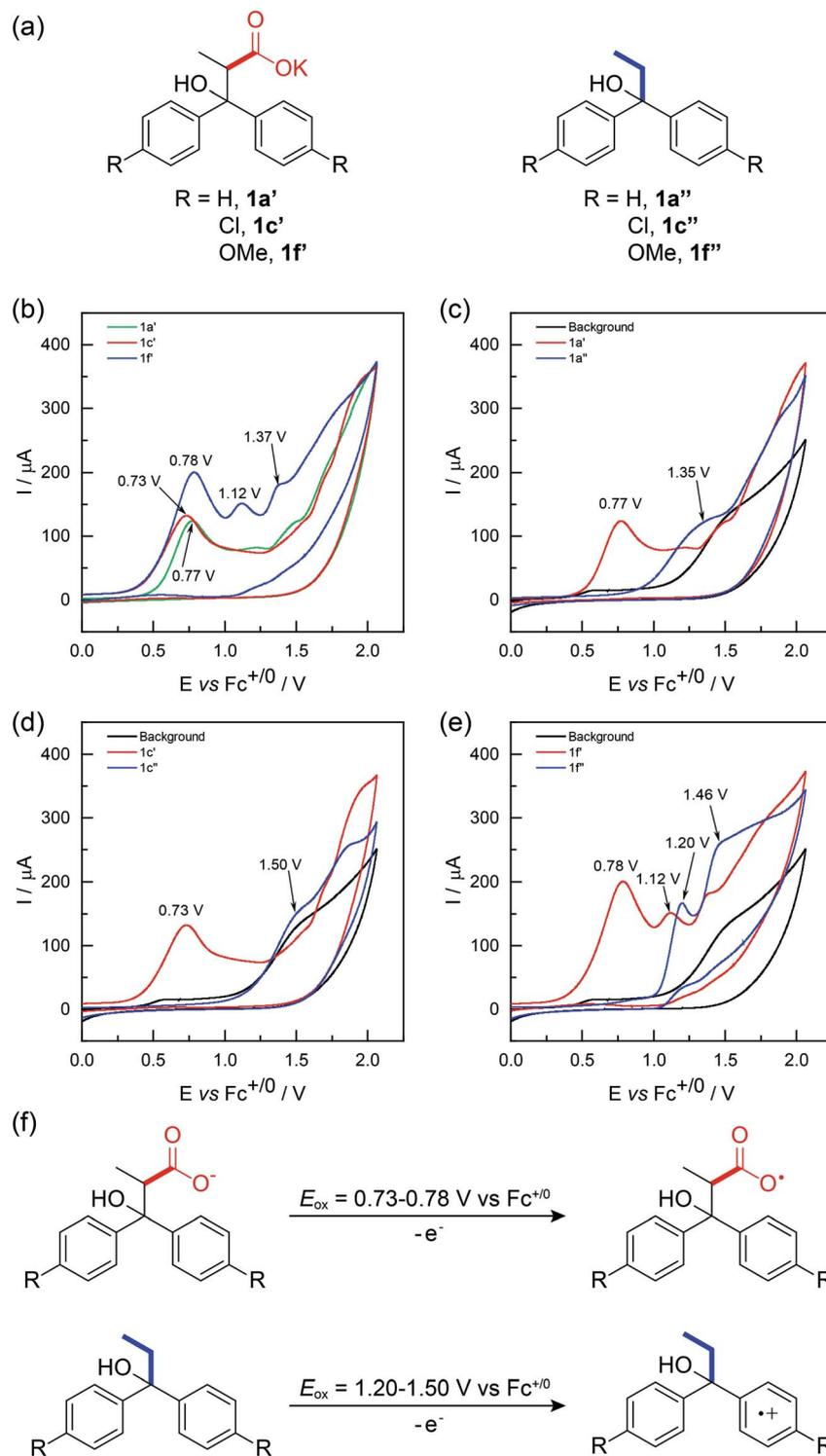
Fig. 1 CV studies: working electrode, platinum disk ( $\phi$  3 mm); counter electrode, silver wire; reference electrode, Ag/AgNO<sub>3</sub> (0.1 M in MeCN); scan rate 0.1 V s<sup>-1</sup>; substrate concentration, 5 mM; background, 0.1 M LiClO<sub>4</sub> in MeCN/H<sub>2</sub>O (3 : 1).
