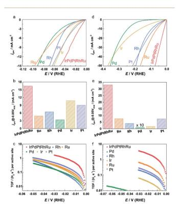
Fig. 4 (a and d) Polarization curves, (b and e) geometric current densities at an overpotential of 50 mV, and (c and f) TOF of IrPdPtRhRu HEA NPs and other monometallic catalysts in (a-c) 0.05 M H<sub>2</sub>SO<sub>4</sub> solution and (d-f) 1.0 M KOH solution
