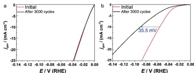
Fig. 5 Comparison of the polarization curves between the initial cycle (red) and after 3000 cycles (black). (a) **IrPdPtRhRu HEA NPs** and (b) commercial Pt/C catalyst. The dashed arrow demonstrates the loss of overpotential at a  $j_{\text{geo}}$  of  $10 \text{ mA cm}^{-2}$ .
