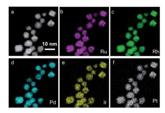
Fig. 1 (a) HAADF-STEM image of IrPdPtRhRu HEA NPs and its corresponding EDX maps showing (b) Ru-L, (c) Rh-L, (d) Pd-L, (c) Ir-L, and (f) Pt-L.
