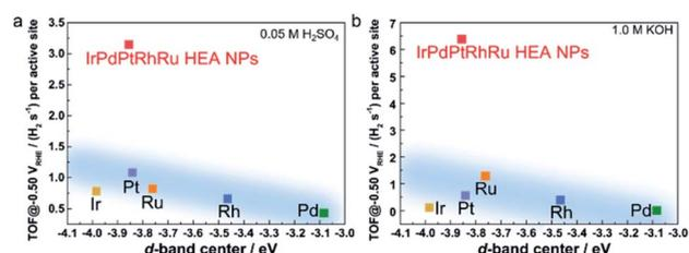
Fig. 6 TOF value at  $-0.05 \text{ V}_{\text{RHE}}$  as a function of the experimental d-band centre of the tested catalysts in (a)  $0.05 \text{ M H}_2\text{SO}_4$  and (b)  $1.0 \text{ M KOH}$  solutions. The d-band centre is relative to the Fermi level. The light blue regions show the trend of the activity following d-band centre theory.
