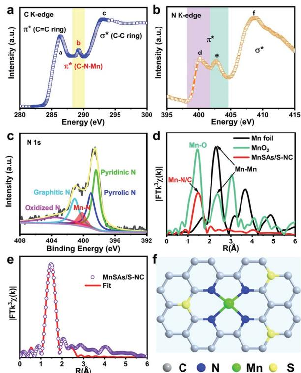
Fig. 2 (a) C K-edge, (b) N K-edge XANES spectra and (c) the N 1s XPS spectra of MnSAs/S-NC. (d) FT  $k^3$ -weighted Mn K-edge EXAFS spectra of MnSAs/S-NC and the references (Mn foil and  $\text{MnO}_2$ ). (e) FT-EXAFS fitting curves of MnSAs/S-NC at the Mn K-edge. (f) Schematic atomic interface model of MnSAs/S-NC.
