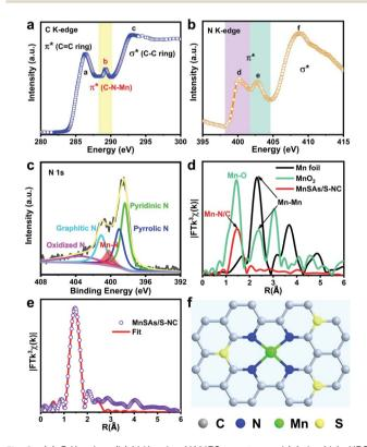
Fig. 2 (a) C K-edge, (b) N K-edge XANES spectra and (c) the N 1s XPS spectra of MnSAs/S-NC. (d) FT  $k^3$ -weighted Mn K-edge EXAFS spectra of MnSAs/S-NC and the references (Mn foil and MnO<sub>2</sub>). (e) FT-EXAFS fitting curves of MnSAs/S-NC at the Mn K-edge. (f) Schematic atomic interface model of MnSAs/S-NC.
