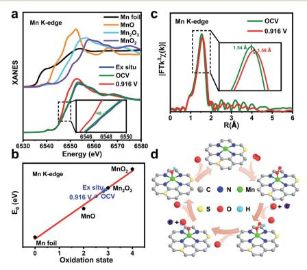
Fig. 4 (a) Operando XANES spectra recorded at the Mn K-edge of MnSAs/S-NC from the OCV condition to 0.916 V during the electrocatalytic ORR. (b) The fitted average oxidation states of Mn from XANES spectra. (c) Mn K-edge EXAFS spectra of MnSAs/S-NC at various potentials during the ORR. (d) The proposed ORR mechanism for the MnSAs/S-NC. C: grey; N: blue; S: yellow; Mn: green; H: cyan; O: red.
