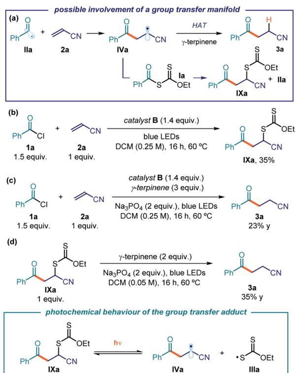
Fig. 12 (a) Focusing on the acyl radical addition step. The model reaction in the presence of a stoichiometric amount of **B** and (b) in the absence or (c) in the presence of  $\gamma$ -terpinene (group transfer conditions). (d) The behavior of group transfer product **IXa** under the reaction conditions and upon blue light irradiation.
