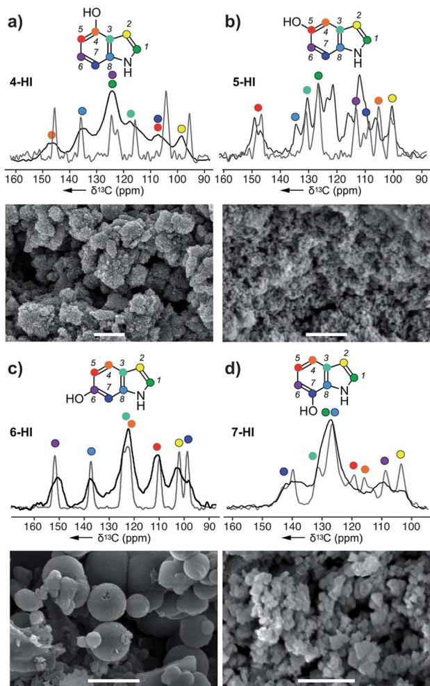
Fig. 3 Melanin particles obtained from the action of *A. bisporus* tyrosinase on (a) 4-HI, (b) 5-HI, (c) 6-HI, and (d) 7-HI. ssNMR spectra of each melanised sample are overlaid with its original monomer, and these peaks were used for assignments. Bars in the SEM images represent 1  $\mu\text{m}$ . Peak assignments are provided in ESI Fig. S9–S12.†
