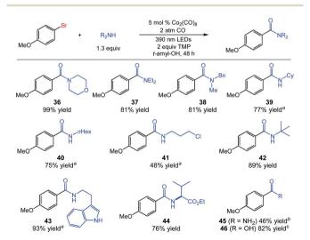
Fig. 3 Cobalt-catalyzed aminocarbonylation of 1-bromo-4-methoxybenzene using diverse amine nucleophiles.  $^a$ Reaction time of 24 h.  $^b$ 10 mol% Co<sub>2</sub>(CO)<sub>8</sub> used as catalyst with ammonium carbamate as nucleophile in the presence of 4 Å molecular sieves.  $^c$ 10 mol% KCo(CO)<sub>4</sub> used as catalyst with 4.0 equiv. of KOH as nucleophile.
