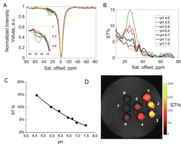
Fig. 2 (A) Z-spectra and (B) ST%-spectra of Eu(HPADO3A) (20 mM) in water at different pH values; (C) ST% effect for Eu(HPADO3A), in water as a function of pH; (D) ST-weighted, CEST map capillaries filled with Eu(HPADO3A) (20 mM) in water at various pH values (1: pH 4.6; 2: pH 5.5; 3: pH 5.9; 4: pH 6.5; 5: pH 6.7; 6: pH 7.0; 7: pH 7.5; 8: water).
