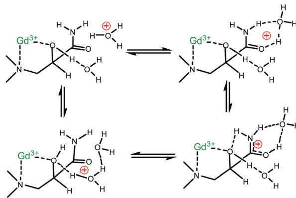
Scheme 2 Mechanism of the H<sup>+</sup> assisted exchange of –OH and –CONH– protons of Gd(HPADO3A). The free rotation around the C2–C3  $\sigma$  bond of the pendant arm guarantees the same mechanism for both enantiomers at C2.
