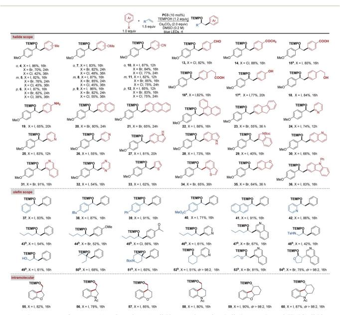
Scheme 3 Reaction scope. General conditions: (hetero)aryl halide (0.30 mmol, 1.0 equiv.), olefin (0.45 mmol, 1.5 equiv.), TEMPOH (0.36 mmol, 1.2 equiv.),  $Cs_2CO_3$  (0.60 mmol, 2.0 equiv.), PC3 (0.03 mmol, 10 mol%), and DMSO (1.5 mL, rigorously degassed by freezing/pumping/thawing). (Hetero)aryl halides and TEMPOH were dissolved in DMSO and added dropwise over 10 h. Isolated yields were reported. <sup>a</sup>With 3 equiv. of  $Cs_2CO_3$ . <sup>b</sup>With 3 equiv. of the olefin.
