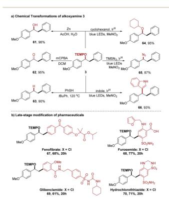
Scheme 4 Synthetic applications of this photocatalytic oxyarylation reaction. (a) Chemical transformations of alkoxyamine 3. (b) Late-stage modification of pharmaceuticals.
