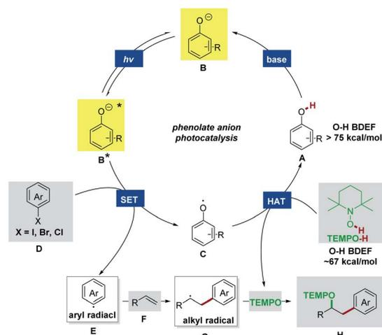
Scheme 2 Proposed photocatalytic mechanism for intermolecular radical oxyarylation.
