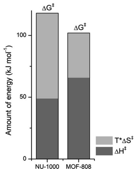
Fig. 7 Contribution of enthalpy (dark grey) and entropy (light grey) terms to the  $\Delta G^\ddagger$  of peptide bond hydrolysis catalyzed by NU-1000 and MOF-808 ( $\Delta G^\ddagger = \Delta H^\ddagger - T\Delta S^\ddagger$  with  $T = 37^\circ\text{C}$  or 310 K, all terms are [kJ mol<sup>-1</sup>]).
