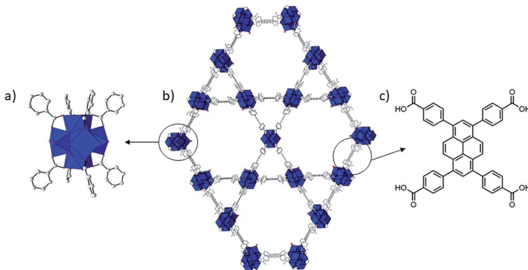
Fig. 1 Structure of NU-1000. Zr = blue coordination polyhedron, O = red, C = gray. H atoms have been omitted for clarity. Zr<sub>6</sub> cluster (a), NU-1000 (b), and TBAPy linker (c).
