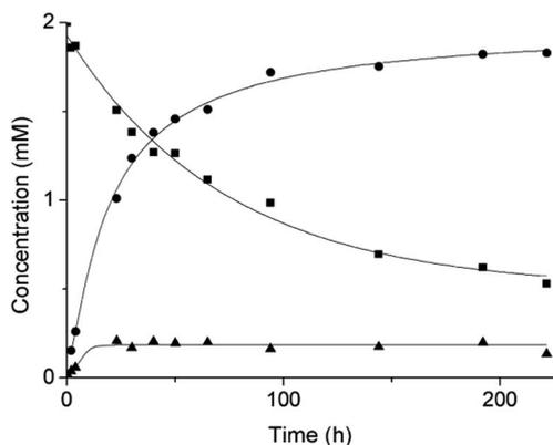
Fig. 3 Reaction of 2 mM GG with 2  $\mu\text{mol}$  NU-1000 at 60  $^{\circ}\text{C}$  and pD 7.4: concentration of GG (squares), G (circles) and cG (triangles) as a function of time by  $^1\text{H}$  NMR.
