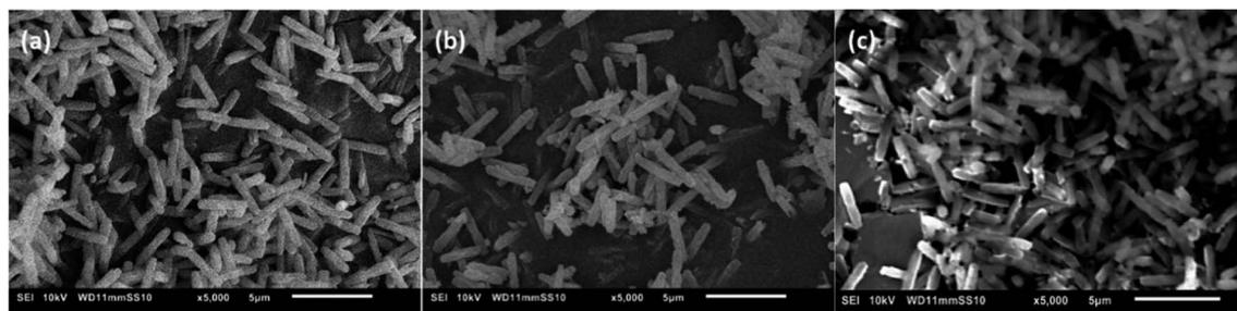
Fig. 5 SEM images of (a) NU-1000 as synthesized, (b) after reaction with 2 mM GG, 60 °C, pH 7.0, 24 h, and (c) after reaction with 0.02 mM HEWL, 60 °C, pH 7.0, 24 h.
