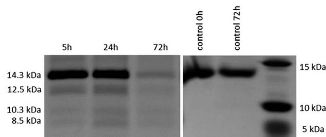
Fig. 4 Silver stained SDS-PAGE gel of HEWL incubated at 60  $^{\circ}\text{C}$  and pH 7.0 in the presence of 2  $\mu\text{mol}$  NU-1000 at different time increments (left); control samples of HEWL incubated at 60  $^{\circ}\text{C}$  and pH 7.0 without NU-1000 (right).
