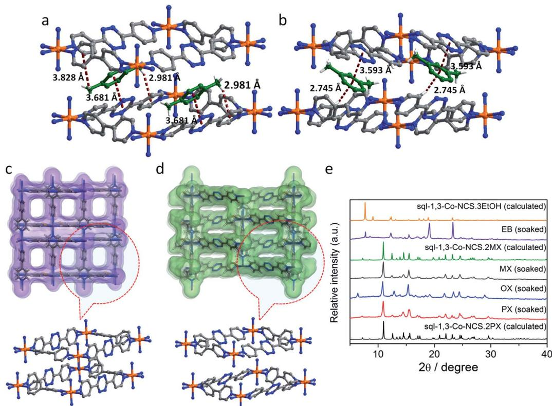
Fig. 6 (a and b) Host–guest interactions in the PX and MX loaded phases, respectively; (c and d) the Connolly surfaces of **sql-1,3-Co-NCS·3EtOH** and **sql-1,3-Co-NCS·2PX** respectively, with a probe radius of 1.4 Å. (e) PXRD patterns for the solvent soaking experiments in pure xylenes and ethylbenzene.
