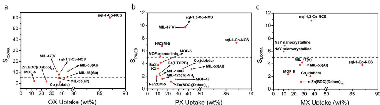
Fig. 5 Comparison of MOMs and zeolites with respect to their (a) OX, (b) PX and (c) MX adsorption capacities and selectivities towards pure xylene isomers vs. EB, respectively.
