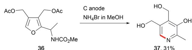
Scheme 18 Electro-conversion of naturally derived furans into pyridoxines, like vitamin B<sub>6</sub>.
