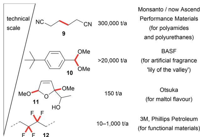
Fig. 2 Some electro-organic processes on the technical scale.
