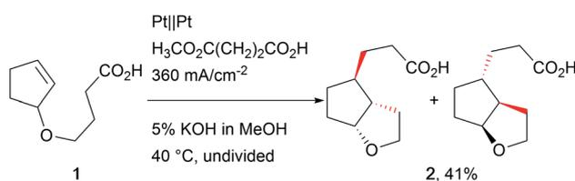
Scheme 1 Kolbe cascade reaction by Schäfer *et al.*
