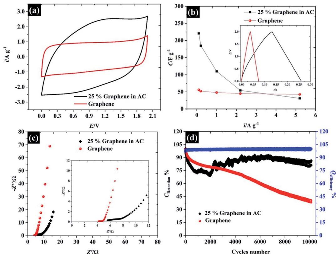
Fig. 9 Performance of supercapacitor devices using 17 M KF electrolyte. (a) CV at  $75 \text{ mV s}^{-1}$ , (b) capacitance and charge/discharge profile at  $2.2 \text{ A g}^{-1}$ , (c) Nyquist plot, and (d) cyclic stability at  $1.0 \text{ A g}^{-1}$  over 10 000 cycles.
