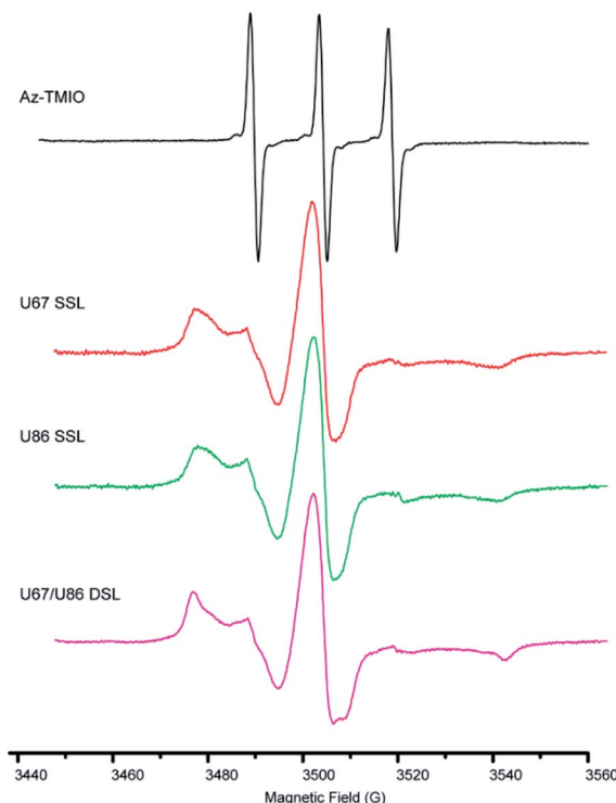
Fig. 3 CW-EPR spectra of the free Az-TMIO (black), the U67 singly spin-labeled (red), U86 singly spin-labeled (green) and U67/U86 doubly spin-labeled (magenta) RNase P samples. All spectra are processed as described in Methods and as shown scaled to the same center-line amplitude. For the RNA spectra, a trace amount of free nitroxide signals ( \leq 0.5\% ) has been subtracted.
