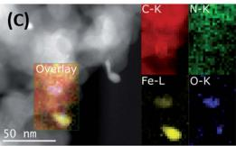
Fig. 2 ADF-STEM images and EELS elemental maps of Fe/Phen@C-800 (A), Fe/Phen@C-800\_S (B) and Fe/Phen@C-800\_R (C).
