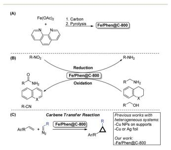
Scheme 1 (A) Preparation of Fe/Phen@C-800, (B) selected known catalytic applications and (C) the present work: cyclopropanation reactions using Fe/Phen@C-800 as the catalyst.
