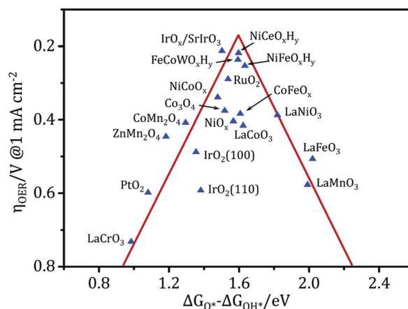
Fig. 7 Activity trends towards the oxygen evolution of (hydro)oxides. The OER overpotential data in the vertical coordinates was measured experimentally and the adsorption energy between two intermediates ( $\Delta G_{\text{O}^*} - \Delta G_{\text{OH}^*}$ ) in the abscissa is the theoretical data calculated using DFT, where all of the data were obtained from the literature.
