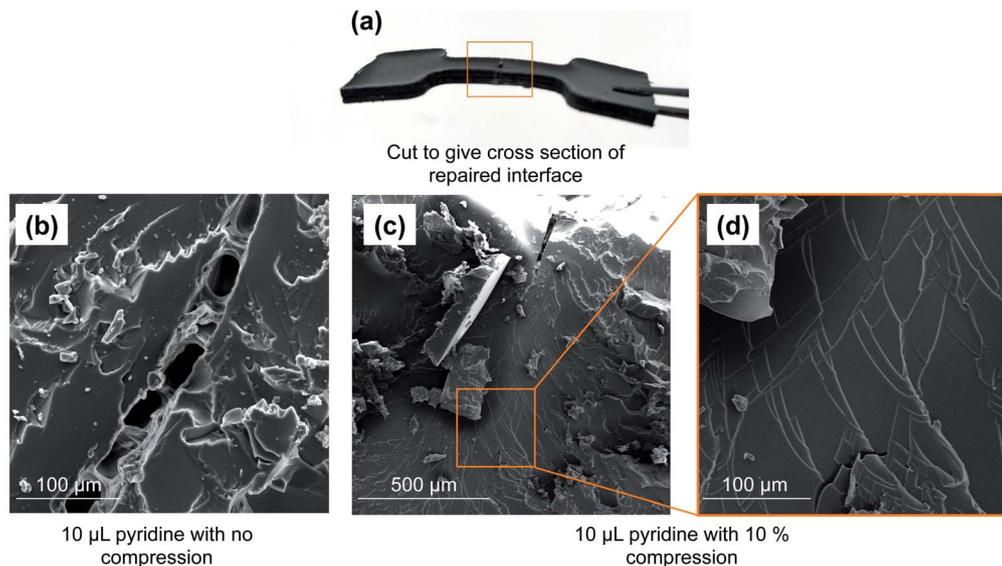
**Fig. 3** (a) Image of repaired polymer. (b) Application of 10  $\mu\text{L}$  of pyridine to a cut polymer interface leads to partial repair when no compression is applied. (c) When pressure is applied to force polymer interfaces together (10% compression, orthogonal to the bonding interfaces), 10  $\mu\text{L}$  of pyridine catalyzes the repair of the polymer. (d) The repaired region of the polymer presents as continuous bulk material.
