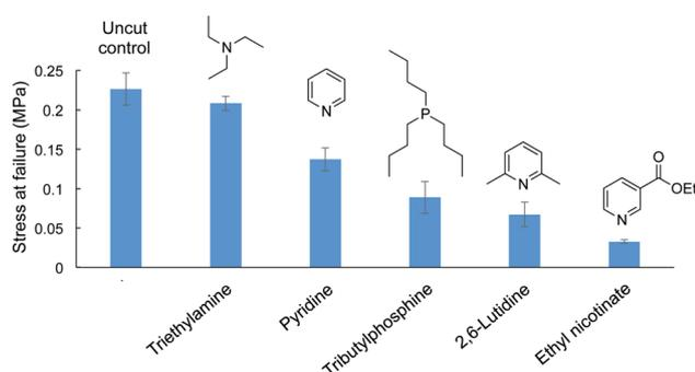
**Fig. 6** Liquid catalysts (10  $\mu$ L) used to repair cut dogbone polymers made by inverse vulcanization (50 wt% sulfur, 35 wt% canola oil, 15 wt% DCPD, sulfur rank  $\sim$  4). Repair with triethylamine returned the dogbone sample to its original tensile strength. All experiments were performed in triplicate.
