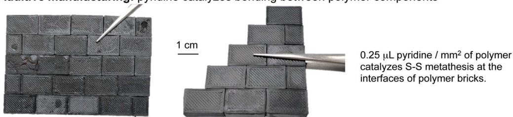
(d) **Repurpose and recycling:** coating ground polymer in pyridine and compressing reshapes polymer
