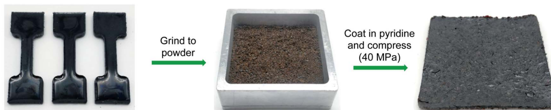
Fig. 7 Applications enabled by pyridine or phosphine catalyzed S-S metathesis on polymers made by inverse vulcanization. (A) Polymer repair. (B) Latent adhesives. (C) Additive manufacturing. (D) Polymer repurposing and recycling.
