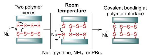
Fig. 1 In this study, nucleophiles such as amines and tributylphosphine were tested in their ability to provoke S–S metathesis between the faces of polymers made by inverse vulcanization.
