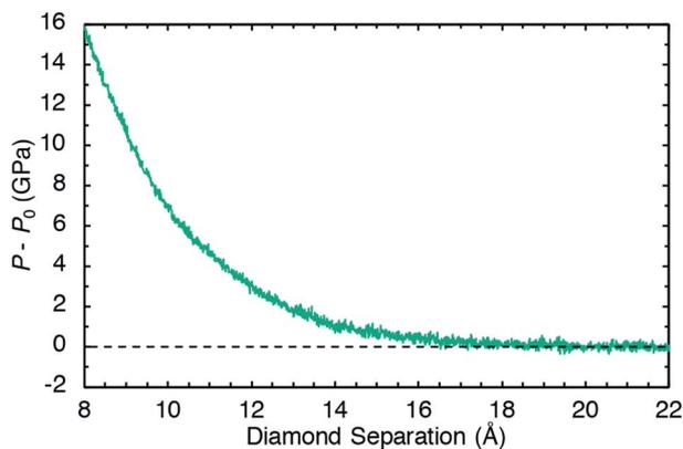
Fig. 2 Pressure as a function of diamond separation distance  $L_z$  measured with respect to a reference  $P_0$  at  $L_z = 22$  Å obtained from an MD simulation where the top diamond rigidly translates at velocity  $V_z = -1.0$  Å ps $^{-1}$ . The pressure is essentially constant for  $L_z \geq 18$  Å.
