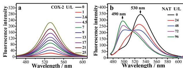
Fig. 1 (a) Emission spectra of 3IAN4 (3.0 μM) with COX-2 (0–25 U L<sup>-1</sup>) in buffer at 25 °C. (b) The emission spectra of 3IAN4 (3.0 μM) with NAT (0–96 U L<sup>-1</sup>) in the presence of acetyl-CoA. 37.5 U L<sup>-1</sup> of COX-2 was first added into solution, which ensured that 3IAN4 fully reacts with NAT.
