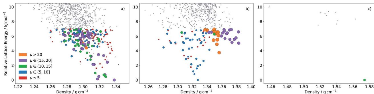
Fig. 10 ESF map of electron mobility in the predicted crystal structures of molecules (a) **4A**, (b) **7A** and (c) **2B**. Each point corresponds to a distinct predicted crystal structure. Colouring and size of the circles correspond to the magnitudes of the calculated mean electron mobilities (in  $\text{cm}^2 (\text{Vs})^{-1}$ ). Grey points are structures above  $7 \text{ kJ mol}^{-1}$ , for which mobilities were not calculated.
