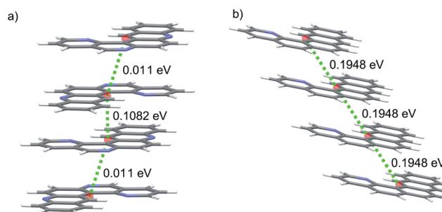
Fig. 9 Coplanar stacking of molecules in the global energy minimum predicted crystal structures of molecules (a) **2A** and (b) **4A**. Red spheres mark the centroids of each molecule. Green dotted lines are the hopping pathways along molecular stacks, showing values of the electronic coupling,  $|V_{\text{ab}}|$ , after scaling.
