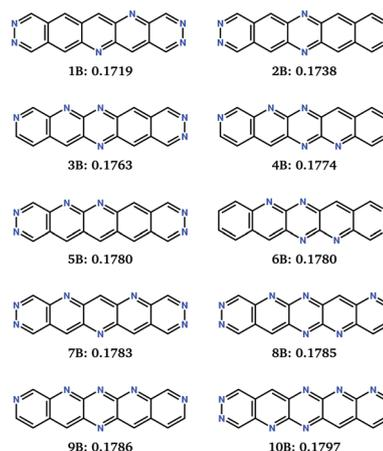
Fig. 8 Chemical diagrams of the top 10 best performing molecules from the combined 10 runs for the evolutionary search for minimisation of fitness function  $F_B$ . Labels and  $F_B$  fitness values (in eV) are given below each chemical diagram.
