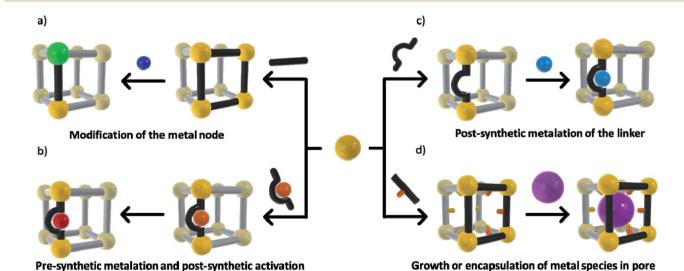
Scheme 1 Matrix isolation methods in MOFs can be achieved via; (a) node related PSM to facilitate attachment of a species, or complete cation metathesis/PSM; (b) PSMet at preinstalled linkers or those unveiled in the MOF post-synthetically; (c) installation of a pre-metalated linker and subsequent chemistry to reveal reactivity; and (d) utilising the pore chemistry to stabilise molecular complexes or subnanometre metal cluster.
