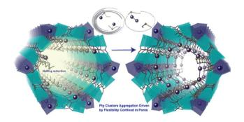
Fig. 10 Detailed comparison of crystal structures of a single pore of the MOFs after the Pt<sup>2+</sup> inclusion (left) and after the reduction process (right) underlining the proposed mechanism to generate the Pt<sub>2</sub> clusters. Reproduced from ref. 182 with permission.
