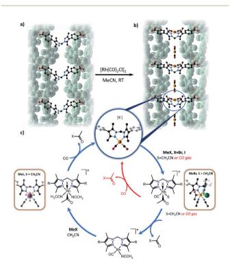
Fig. 7 Metalation of MnMOF-1 (a) with [Rh(CO)<sub>2</sub>Cl]<sub>2</sub> yields MnMOF-1 [Rh(CO)<sub>2</sub>][Rh(CO)<sub>2</sub>Cl<sub>2</sub>] (b). The proposed catalytic cycle for the carbonylation of methyl iodide using the Rh(ı) functionalised MOF is depicted (c) for both the gas phase (red) and solution phase (blue). R =MOF framework (MOF backbone - green surface, C - black, N lavender, O - red, Rh - orange, I - green).
