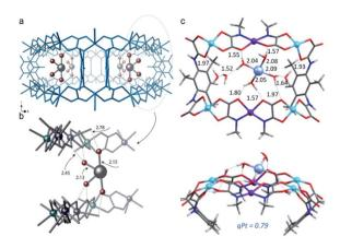
Fig. 11 (a and b) Detailed SC-XRD results of the  $Pt_1^{1+}$  complex within the MOF. (c) DFT optimized structure of the  $Pt_1^{1+}$  complex with seven water molecules. Reproduced from ref. 183 with permission.
