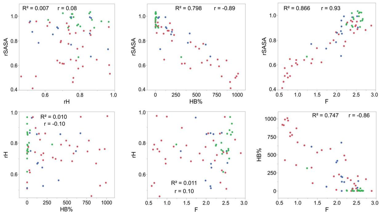
Fig. 4 2D-scatter plots of the molecular descriptors proposed for predicting supramolecular gelation for the complete dataset. The points are coloured according to their outcome of the gelation test (S = green, G = blue and P = red). The Pearson correlation coefficient ( $r$ ) and the coefficient of determination ( $R^2$ ) between two descriptors are provided as well.
