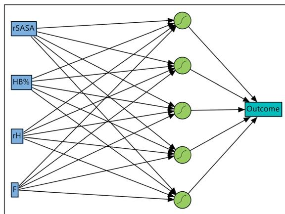
**Fig. 7** Optimized artificial neural network consisting out of the input layer, a hidden layer having 5 sigmoid neurons and the output layer.
