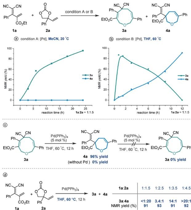
**Scheme 4** Control experiments. (a) Reaction progress was monitored in MeCN at 20 °C; (b) Reaction progress was monitored in THF at 60 °C; (c) Transformation from 3a to 4a; (d) Effect of the loading of VEC on the regioisomeric ratio.
