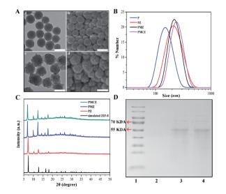
Fig. 1 Characterization of the PDAs-MB-CAT-ZIF-8 (PMCZ) nanoparticles. (A) TEM and SEM images of PDAs (a, b) and PMCZ (c, d), respectively. Scale bar, 100 nm. (B) Size distributions of PDAs (P), PDAs-ZIF-8 (PZ), PDAs-MB-ZIF-8 (PMZ) and PMCZ nanostructures. (C) XRD patterns of the simulated ZIF-8, PZ, PMZ and PMCZ nanohybrids. (D) SDS-PAGE analysis of the corresponding protein from marker (1), PMZ (2), PMCZ (3) and free catalase (CAT, 4).
