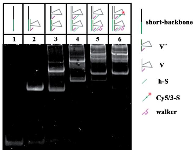
Fig. 2 Native PAGE (8%) images: lane 1, short-backbone (0.3  $\mu$ M); lane 2, short-backbone + V'' (0.3  $\mu$ M); lane 3, short-backbone + V'' + V (0.3  $\mu$ M); lane 4, short-backbone + V'' + V + h-S (0.3  $\mu$ M); lane 5, short-backbone + V'' + V + h-S + walker (0.3  $\mu$ M); lane 6, short-backbone + V'' + V + Cy5/3-S + walker (0.3  $\mu$ M).
