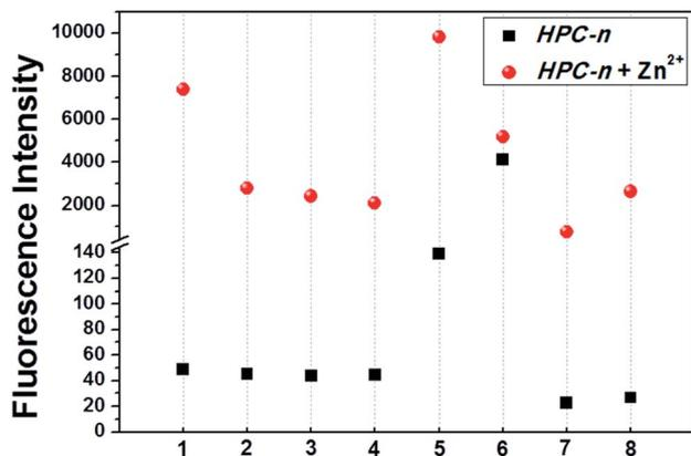
Fig. 2 The intensities of the fluorescence background (black squares) and reporting experiment (red circles) signals for HPC-*n* (*n*: 1–8) (1  $\mu$ M) in response to Zn ions (20  $\mu$ M). All experiments were performed in HEPES buffer solution (50 mM HEPES, 100 mM KNO<sub>3</sub>, pH = 7.2).
