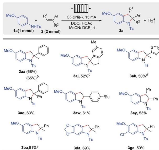
**Scheme 4** Substrate scope in the electrochemical flow cell. <sup>a</sup> Reaction conditions:  $I$  = 10 mA, **1a** (1.0 mmol), **2** (2.0 mmol), 5 mol% DDQ, solvent (MeCN/DCE = 10/5 mL), in the electrochemical flow cell, nitrogen, and 8 h. Isolated yields are shown. <sup>b</sup> 4 mmol scale, MeCN/DCE (50 mL/25 mL). <sup>c</sup> 10 h. <sup>d</sup> 8 mA, 10 h. <sup>e</sup> 8 mA, and 5 h.
