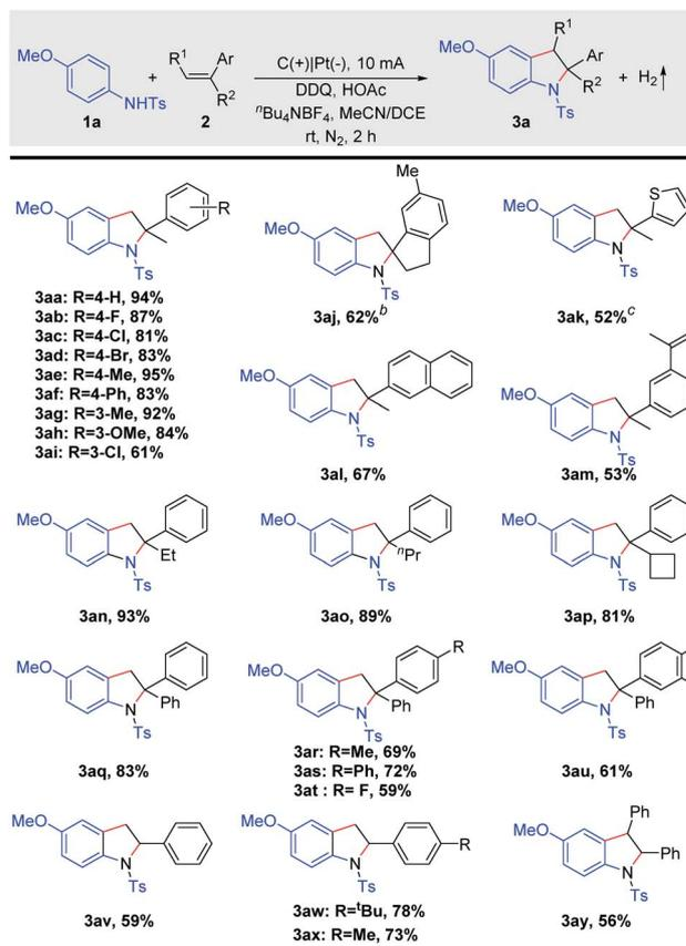
Scheme 2 Substrate scope of alkenes.<sup>a</sup> <sup>a</sup> Reaction conditions: carbon rod anode ( $\phi$  6 mm), Pt plate cathode (15 mm  $\times$  15 mm  $\times$  0.3 mm), constant current = 10 mA, **1a** (0.20 mmol), **2** (0.40 mmol), HOAc (0.20 mmol), 10 mol% DDQ, solvent (MeCN/DCE = 4/2 mL), undivided cell, nitrogen, and 2 h (3.7 F mol<sup>-1</sup>). Isolated yields are shown. <sup>b</sup> 4 h. <sup>c</sup> 8 mA, and 3 h.
