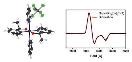
Fig. 3 (Left) X-ray crystal structure of 3. Atoms are shown at the 50% probability level. A non-coordinated pyridine has been omitted for clarity. (Right) Experimental (black) and simulated (red) EPR spectra of 3 in  $CH_2Cl_2$ /pyridine at  $-80\,^{\circ}C$ .
