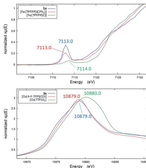
Fig. 4 Top: Fe pre-edge peaks in the XANES spectra of **1a** (blue),  $[\text{Fe}(\text{TPFPP})(\text{CPh}_2)]$  (red), and  $[\text{Fe}(\text{TPFPP})\text{Cl}]$  (green). Bottom: Os L<sub>3</sub>-edge peaks in the XANES spectra of **3a** (blue),  $[\text{Os}(4\text{-F-TPP})(\text{CO})]$  (red), and *trans*-dioxo complex  $[\text{Os}(\text{TTP})\text{O}_2]$  (green).
