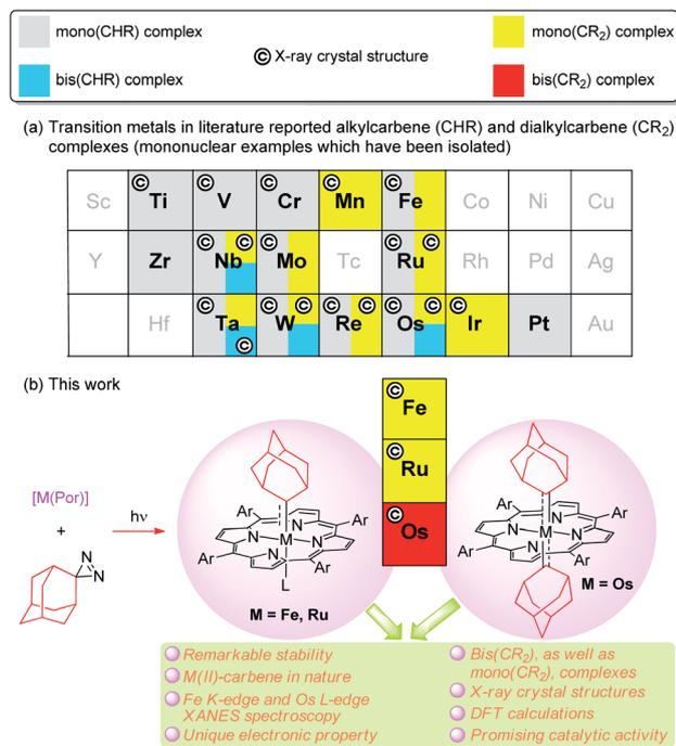
Fig. 1 (a) Literature examples of isolated mononuclear (di)alkylcarbene complexes of TMs. Mono- and bis(CHR/CR<sub>2</sub>) complexes are represented by different colors filled. Structurally characterized examples are indicated by ⊙. TMs for which no isolated examples were found are left blank. (b) Group 8 metal porphyrin dialkylcarbene complexes reported in this work. M≡Ad (M = Fe, Ru, Os) represents an Ad → M σ bonding (–) and a M → Ad π-backbonding (---).
