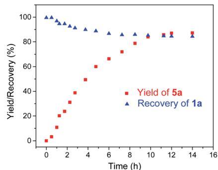
Fig. 11 Time course plot of the reaction among  $\text{Ph}_2\text{CN}_2$ , styrene, and **1a** during <sup>1</sup>H NMR monitoring.
