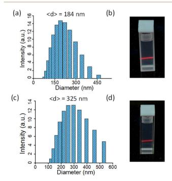
Fig. 2 The size distribution from DLS measurements of dispersed nanosheets (a) L·Eu and (c) L·Tb in chloroform—tetrahydrofuran (1:1, v/v). Photograph of (b) L·Eu and (d) L·Tb nanosheets dispersed in chloroform—tetrahydrofuran (1:1, v/v) showing a strong Tyndall scattering.
