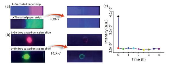
Fig. 8 (a) Visual color change of L·Eu and L·Tb coated paper strips upon addition of FOX-7 under UV light irradiation ( $\lambda_{ex} = 352$  nm). (b) Visual color change of L·Eu and L·Tb nanosheets drop-cast on a glass slide upon addition of FOX-7 under UV light irradiation ( $\lambda_{ex} = 352$  nm). (c) The plot of emission intensity of the L·Tb nanosheet dispersion in MeCN (2 mg/2 mL) in the presence of FOX-7 (100  $\mu$ M) with varying the incubation time.
