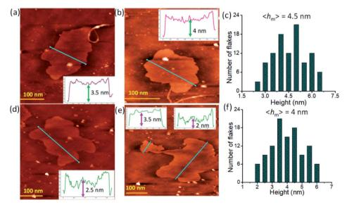
Fig. 4 AFM topography (height) scanning images of randomly distributed nanosheets of (a and b)  $L \cdot Eu$  and (d and e)  $L \cdot Tb$  deposited on a silicon wafer. Inset: height profiles of nanosheets of  $L \cdot Eu$  and  $L \cdot Tb$  extracted along the lines drawn in panels (a), (b), (d) and (e). (c and f) The statistical height distribution of  $L \cdot Eu$  and  $L \cdot Tb$  nanosheets based on AFM investigations.
