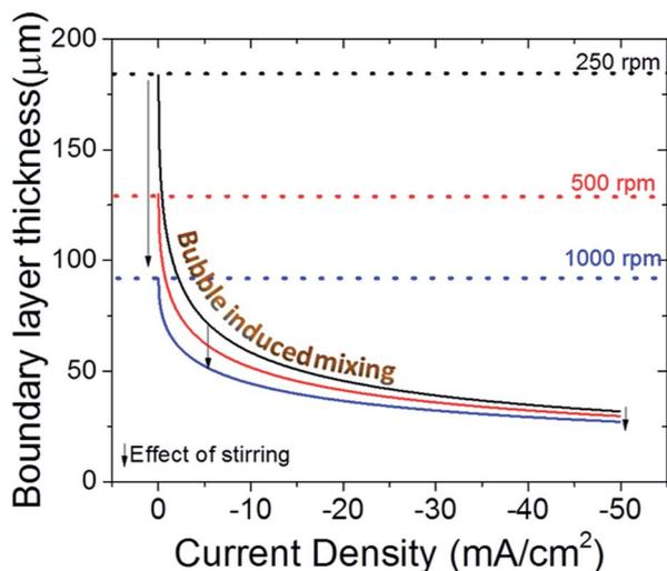
Fig. 6 Effect of stirring and bubble formation on boundary layer thickness for  $\text{CO}_2(\text{aq})$ . The effect of magnetic stirring is represented by the dashed lines and arrows. Note that effect of stirring on the boundary layer thickness will strictly depend on the cell design. Reynold's numbers are assumed to be 100, 200 and 400 for increasing stirring rates. The bubble induced mixing changes as a function of current density.
