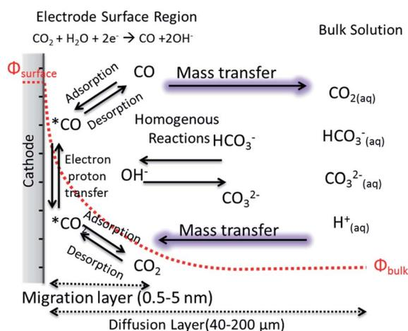
Fig. 3 A schematic description for electrochemical CO<sub>2</sub> reduction composed of electrode surface region, mass transport layer and bulk solution.
