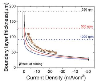
Fig. 6 Effect of stirring and bubble formation on boundary layer thickness for  $\rm CO_2$ (aq). The effect of magnetic stirring is represented by the dashed lines and arrows. Note that effect of stirring on the boundary layer thickness will strictly depend on the cell design. Reynold's numbers are assumed to be 100, 200 and 400 for increasing stirring rates. The bubble induced mixing changes as a function of current density.
