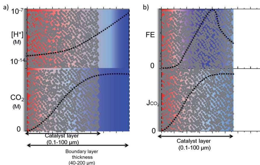
Fig. 5 Schematic description of the (a) concentration gradient for protons and  $\text{CO}_{2(\text{aq})}$  along the catalyst layer in  $\text{CO}_2$  saturated aqueous solutions (b) selectivity and activity gradient along the catalyst layer is represented by FE and partial current density of electrochemical  $\text{CO}_2$  reduction products. Blue and red colour represents high and low values, respectively. (Dashed lines only as guide to eye).
