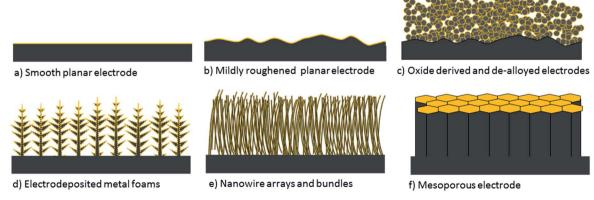
Fig. 1 Depiction of 2-D planar and commonly used 3-D nanostructured and mesostructured electrodes. Yellow colour represents the ECSA.
