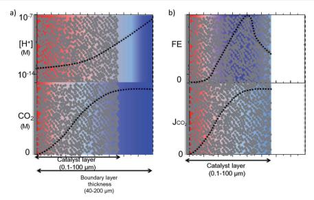
Fig. 5 Schematic description of the (a) concentration gradient for protons and  $CO_{2(aq)}$  along the catalyst layer in  $CO_2$  saturated aqueous solutions (b) selectivity and activity gradient along the catalyst layer is represented by FE and partial current density of electrochemical  $CO_2$  reduction products. Blue and red colour represents high and low values, respectively. (Dashed lines only as quide to eye).
