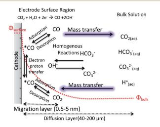
Fig. 3 A schematic description for electrochemical CO2 reduction composed of electrode surface region, mass transport layer and bulk solution.
