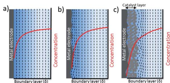
Fig. 4 Schematic description of the diffusion front and concentration profiles, *e.g.* pH, for different electrode morphologies (a) flat smooth surface (b) flat roughened surface (c) rough 3-D porous electrode.
