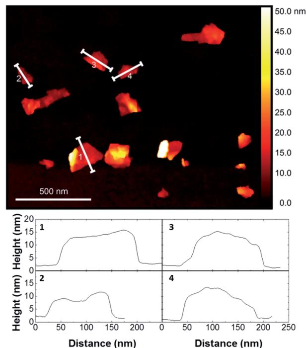
Fig. 4 Representative AFM image of graphene flakes prepared with pyrene cation **10b** and cross-section analyses of several flakes. See ESI† for AFM images of graphene flakes exfoliated with all pyrene cations.
